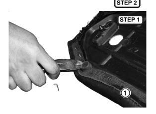
**STEP 2:** Carefully peel the stock cover ② back off the seat's foam ③. In some cases the cover may be glued or bonded to the foam, so the foam may lift off the pan without having to separate the cover from the foam. If this is the case, move on to STEP 4. Other wise, once the cover is removed from the foam, move to STEP 3.
