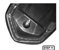
**STEP 12:** Make sure you do not cover bumpers or tabs with the cover. This could prevent the seat from properly mounting to your motorcycle. Route the cover ① carefully around these features on the seat.
